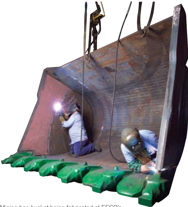
Mining hoe bucket being fabricated at ESCO's Phoenix facility.
