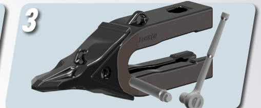
3 Insert Helical Pin and Rotate 180 degrees with Socket Wrench to Engage Lock
