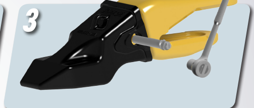
3 Insert Helical Pin & Rotate 180 degrees with Socket Wrench to Engage Lock
